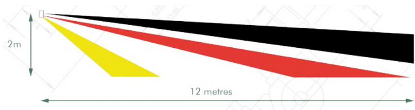
Typical Field of View diagrams when used in conjunction with type A pyro
