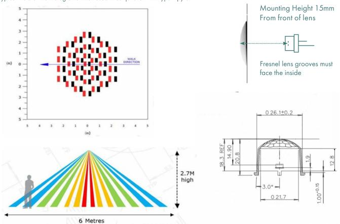
Note: Field of view (FOV) diagrams are idealised. Exact zones may depend on mounting conditions, detector type etc. FOV diagrams have been raytraced in reverse, i.e. from detector to the floor.
